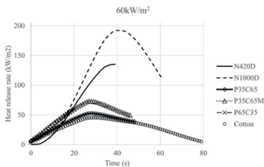
Figure 10: HRR curves at 60kW/m<sup>2</sup> heat flux.
