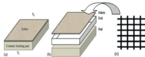
**Figure 2:** Sample positioned over the backing pad for the cone test (a). Sample assembly (b). (Tata et al., 2011), metal grid (c).
