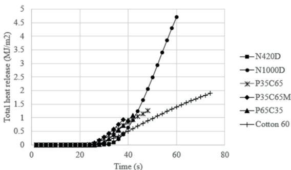
Figure 14: Total heat release of fabric tested at 60 kW/m<sup>2</sup>.
