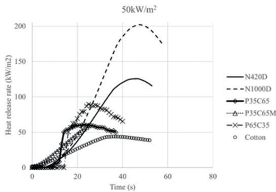
Figure 9: HRR curves at 50kW/m<sup>2</sup> heat flux.
