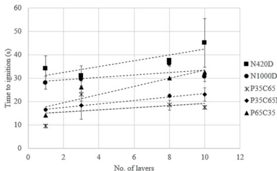
Figure 6: Time to ignition vs. number of fabric layers.
