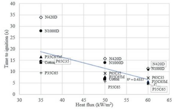
Figure 7: TTI vs. heat flux.
