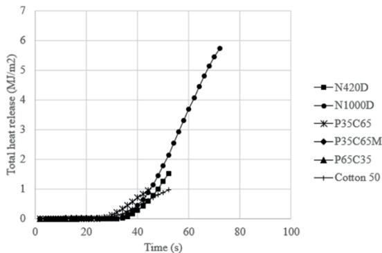
Figure 13: Total heat release of fabric tested at 50 kW/m<sup>2</sup>.
