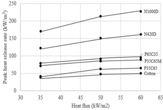
Figure 11: PHRR vs heat flux
