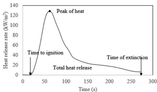
**Figure 3:** Typical heat release rate versus time curve based on kenaf fabric tested at 35 kW/m<sup>2</sup>.
