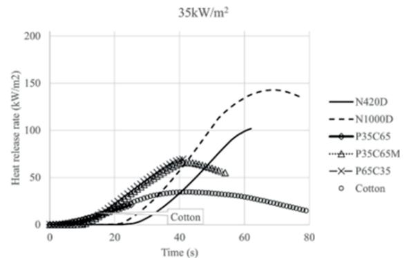
Figure 8: HRR curves at 35kW/m<sup>2</sup> heat flux.
