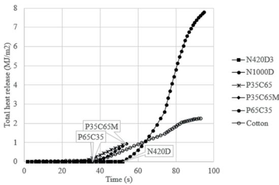
Figure 12: Total heat release of fabric tested at 35 kW/m<sup>2</sup>.
