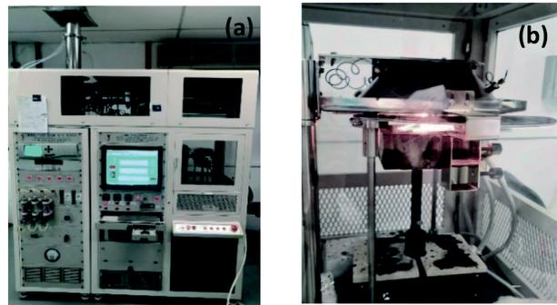
**Figure 1:** Cone calorimeter (Chee et al., 2020).
